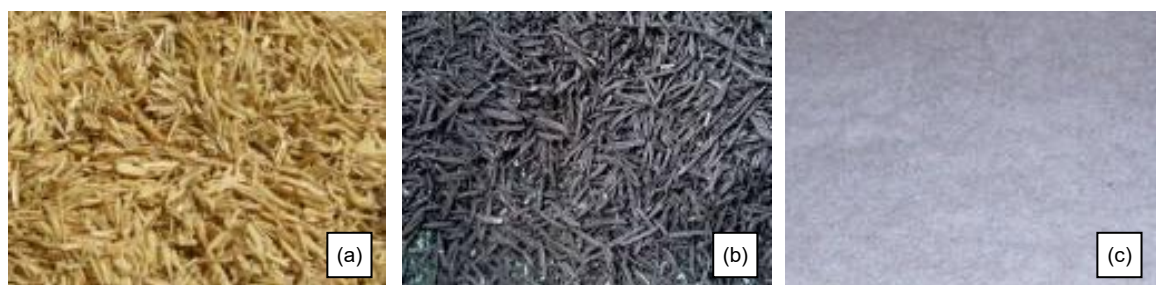
Figure 1 (a) Rice Husk (RA) (b) Rice Husk Ash (RHA) (c) White Rice Husk Ash (WRHA)
