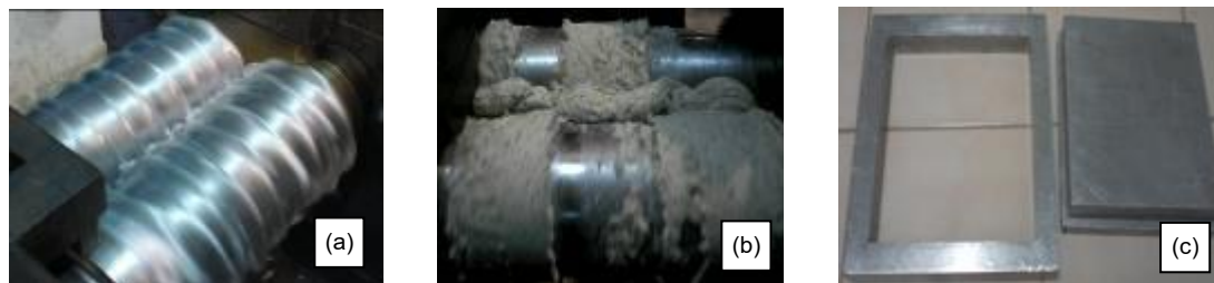
Figure 2 (a) Two roll mill (b) Two roll mill operation of PVC/DINP/WRHA (c) Stainless steel mold
